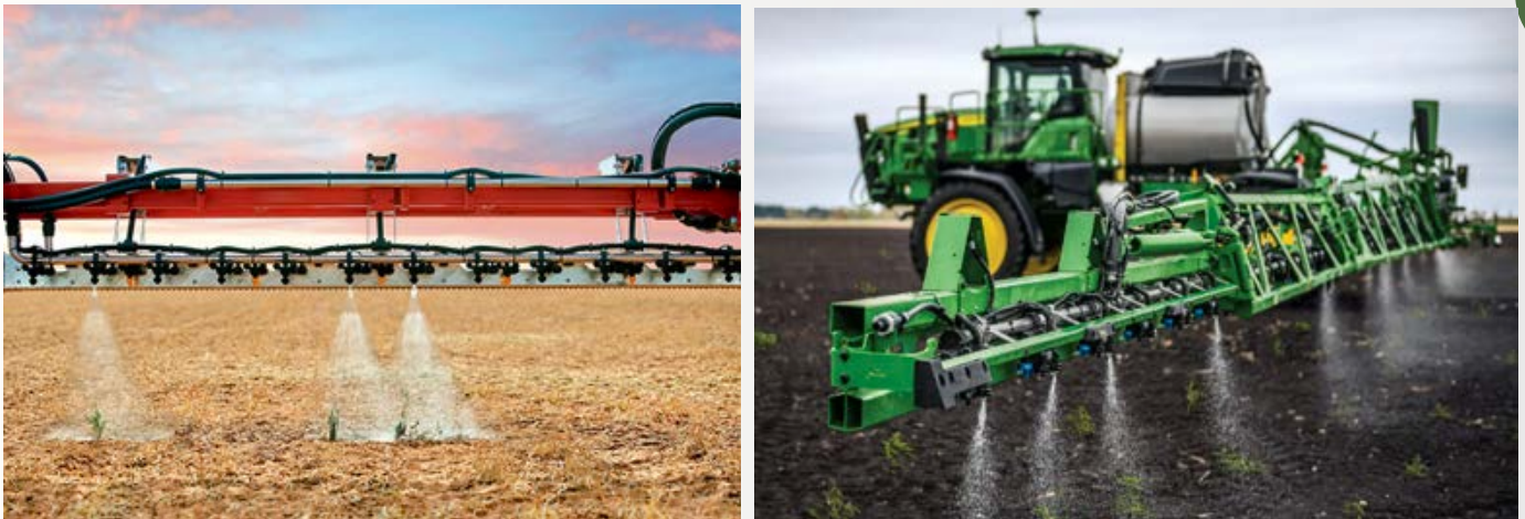
Figure 3.31. Spot-spraying with weed detection
