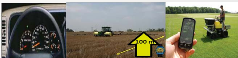
Figure 3.13. Steps of Forward Speed Measurement
