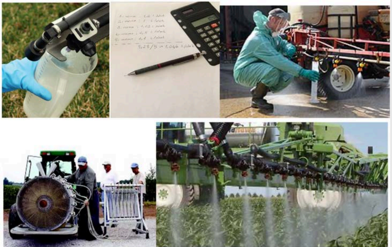
Figure 3.16. Measurement of Nozzle Flow Rate
