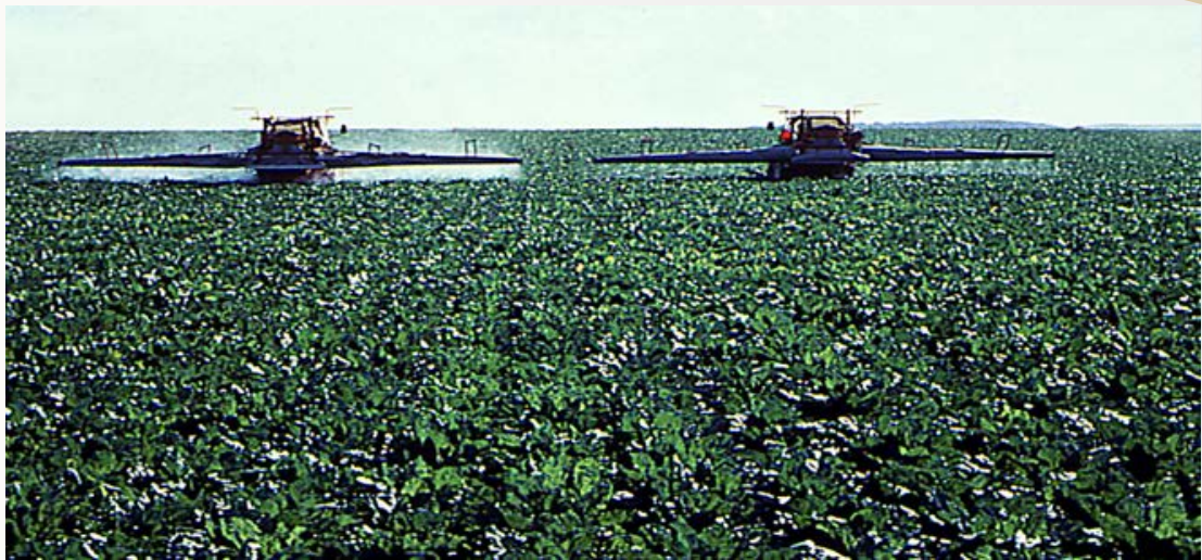
Figure 3.20. Effect of air assistance (Hardi)
