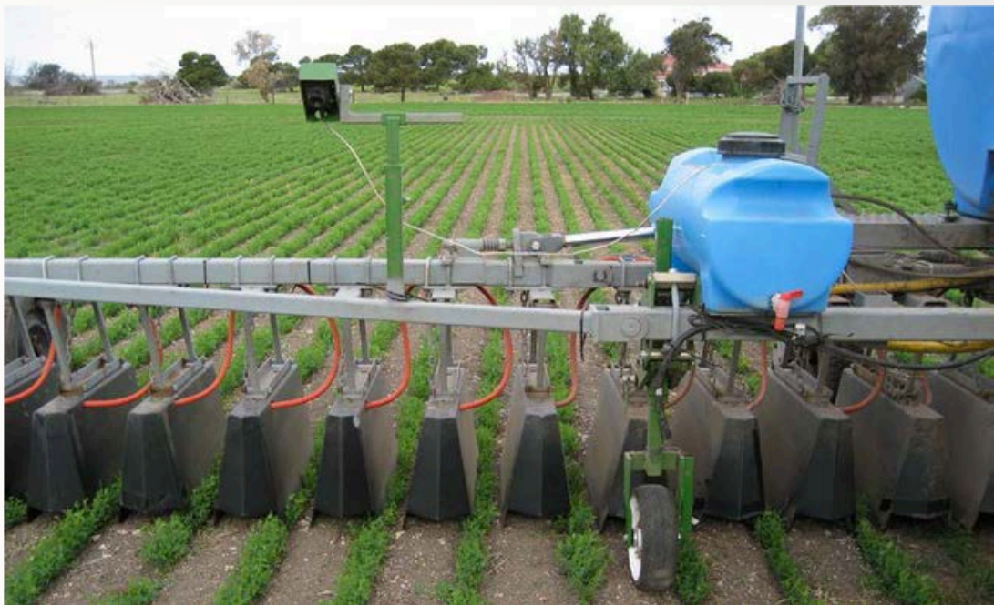
Figure 3.28. Shielded sprayer for field crops (a) in wider row spacings (b) in narrower row spacing
