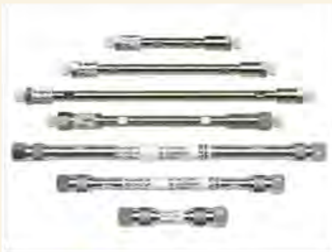
Figure 4. Columns for HPLC, from Agilent manufacturer, of different sizes ( https://www.agilent.com/ )
