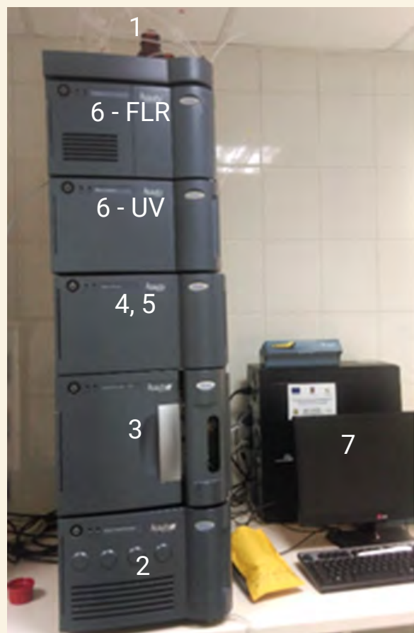
Figure 3 -2 Waters ACQUITY UPLC chromatograph (Waters, Milford, MA) equipped with UV-PDA and FLR detectors
