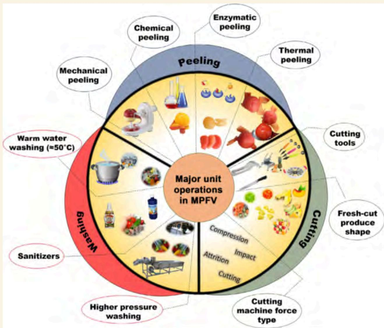
Figure 6. Major operation units used in minimal processing of fruits and vegetables (MPFV)
